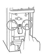
**5** Fix the printed circuit board located in the unit and the conversion board, with an attached screw.
