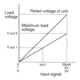
■ When the maximum load current and the rated current of CT1 Are the same, and when the maximum load voltage and the rated voltage of PT are the same
