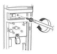
**6** After checking to see that the conversion board is properly installed, and that the screw is fastened tightly, attach the cover.
