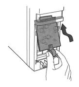
**3** Connect the connectors "CN2" and "CN3" which are located on the conversion board to the connectors "CN2" and "CN3" which are located at both sides of the printed circuit board in the unit.
