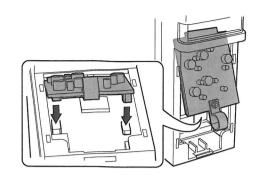
**4** After connecting them, lightly push the area of the connectors "CN2" and "CN3" located on the conversion board with the index finger. You should hear it click at that moment.
