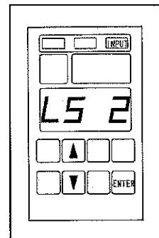
Priority settings changed by manipulating the signal display panel as an example, UF-CL signals can change the settings.
