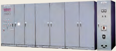
Power supply for plasma arc generation
