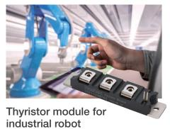
The power supplies for servo motors used in industrial robots are frequently turned ON / OFF, so our durable packages adopting transfermold process are used by many customers. It has been well received by customers especially seeking compactness.
