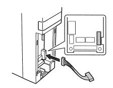
3 Insert another end of the cable into a connector "CN1" which is located on the display panel. The connector has a polarity. When inserting the cable, align a projecting part on the cable and a groove onto the connector.
