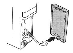
4 In place of the cover which was removed in the procedure "1" above, install the display panel on the front of the unit.
