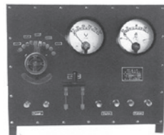
Choke coil auto transformer
