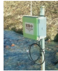
Monitoring the level of the river water, the water level gauge in the photo incorporates the general-purpose transmitter circuit board.
